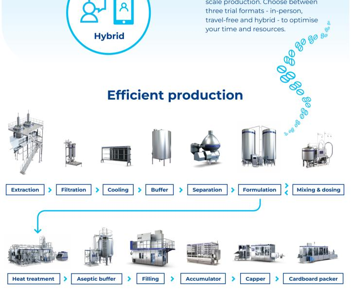
All our processing lines are designed to ensure the highest standards of quality, safety and efficiency. They reduce total cost of ownership while being easy to maintain and service. Togther we can design and build the optimal production line, or simply adapt your existing line to enable RTD coffee production. As a third option, we can help you find a suitable co-manufacturer in your region.
